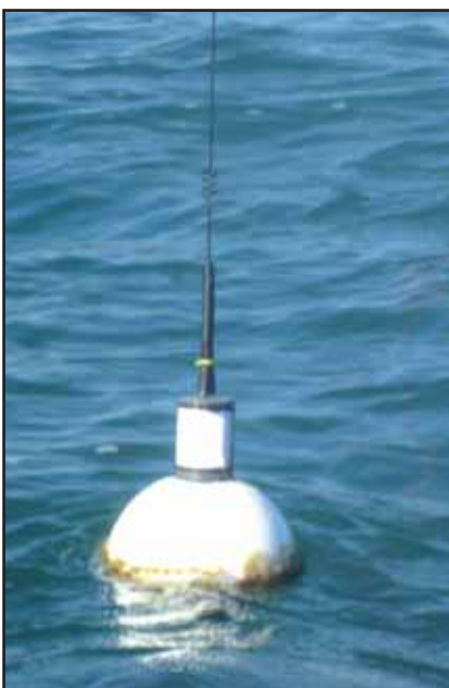
Picture of surface buoy with RF module and antennae.
