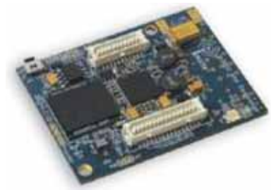
Figure 2. Rowden White Sensor Networking Laboratory is to be equipped with 100 Imote2 nodes from Crossbow
